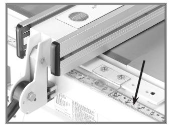
Figure 15. Scale installed on front rail.
